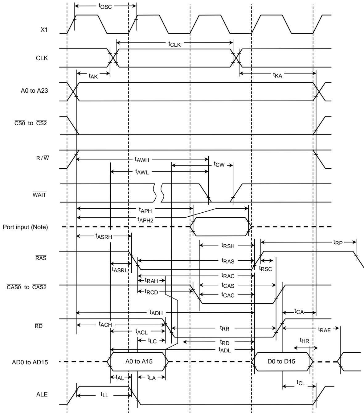
Note: Since the CPU accesses the internal area to read data from a port, the control signals of external pins such as  $\overline{RD}$  and  $\overline{CS}$  are not enabled. Therefore, the above waveform diagram should be regarded as depicting internal operation. Please also note that the timing and AC characteristics of port input/output shown above are typical representation. For details, contact your local Toshiba sales representative.
