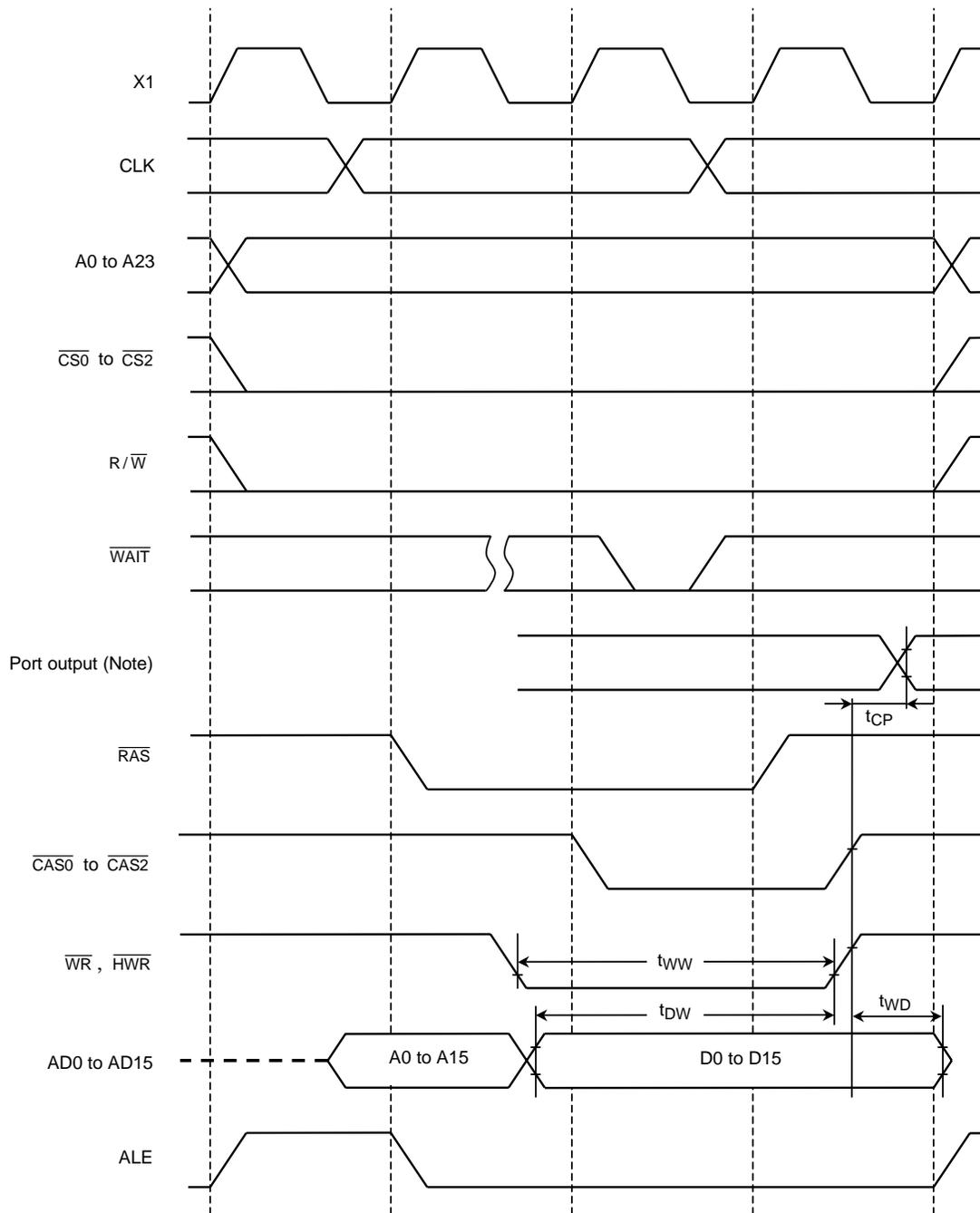
Note: Since the CPU accesses the internal area to write data to a port, the control signals of external pins such as  $\overline{WR}$  and  $\overline{CS}$  are not enabled. Therefore, the above waveform diagram should be regarded as depicting internal operation. Please also note that the timing and AC characteristics of port input/output shown above are typical representation. For details, contact your local Toshiba sales representative.
