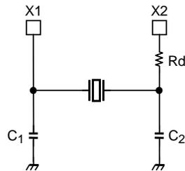
Figure 1 Example of High Frequency Resonator Connection
