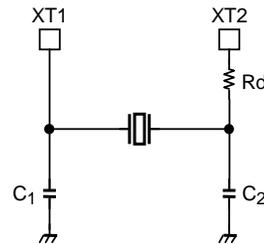
Figure 2 Example of Low Frequency Resonator Connection
