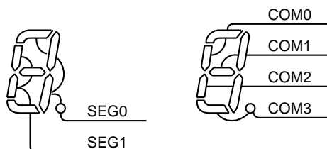
Figure 13-6 Example of COM, SEG Pin Connection (1/4 Duty)
