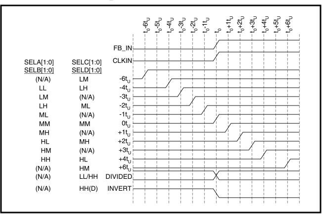
FIGURE 3. TYPICAL OUTPUTS WITH FB IN CONNECTED TO A ZERO-SKEW OUTPUT
