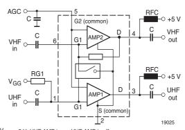
$V_{GG} = 5 \text{ V: UHF AMP is on; VHF AMP is off}$   $V_{GG} = 0 \text{ V: UHF AMP is off; VHF AMP is on}$ (0 = shorted to Ground or open)
