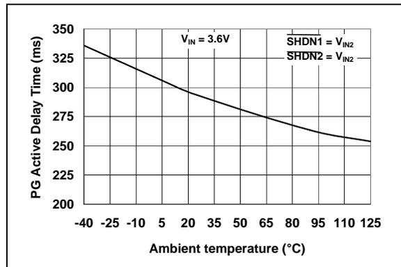
**FIGURE 2-29:** PG Active Delay Time-out vs. Ambient Temperature.
