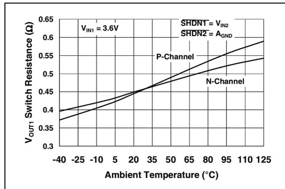
**FIGURE 2-17:** Buck Regulator Switch Resistance vs. Ambient Temperature.
