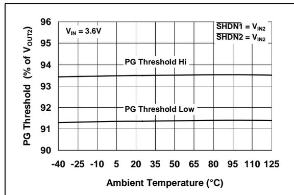
**FIGURE 2-30:** PG Threshold Voltage vs. Ambient Temperature.
