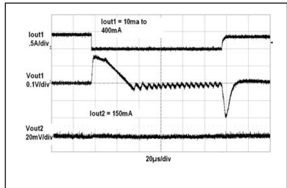
**FIGURE 2-35:**  $V_{OUT1}$  Load Step Response vs. Time.
