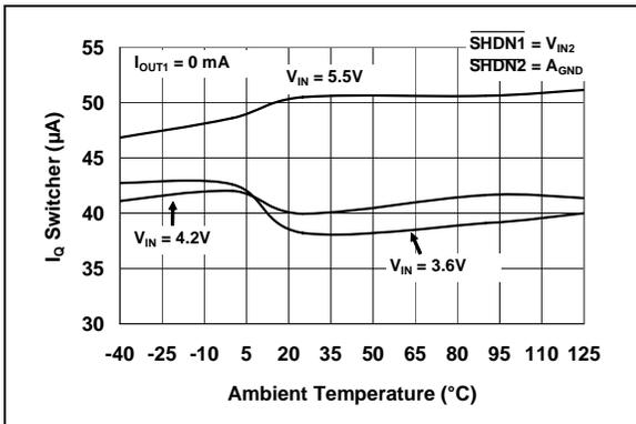
**FIGURE 2-2:**  $I_Q$  Switcher Current vs. Ambient Temperature.
