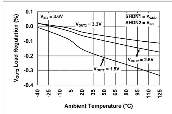
**FIGURE 2-28:**  $V_{OUT2}$  Load Regulation vs. Ambient Temperature.
