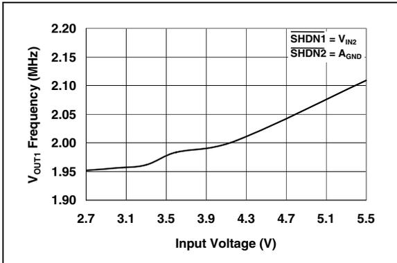
**FIGURE 2-13:**  $V_{OUT1}$  Switching Frequency vs. Input Voltage.
