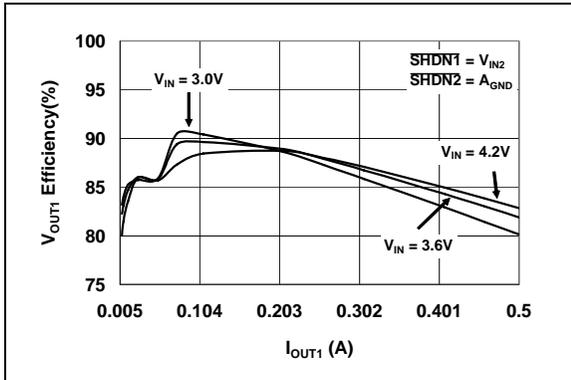
**FIGURE 2-7:**  $V_{OUT1}$  Output Efficiency vs.  $I_{OUT1}$  ( $V_{OUT1} = 1.8V$ ).
