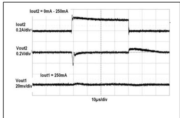
**FIGURE 2-36:**  $V_{OUT2}$  Load Step Response vs. Time.
