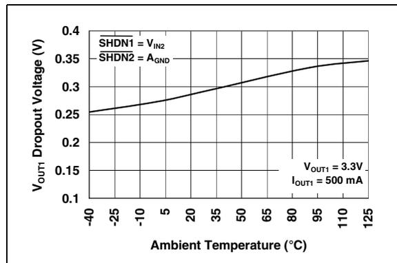
**FIGURE 2-18:**  $V_{OUT1}$  Dropout Voltage vs. Ambient Temperature.
