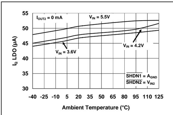
**FIGURE 2-3:**  $I_Q$  LDO Current vs. Ambient Temperature.
