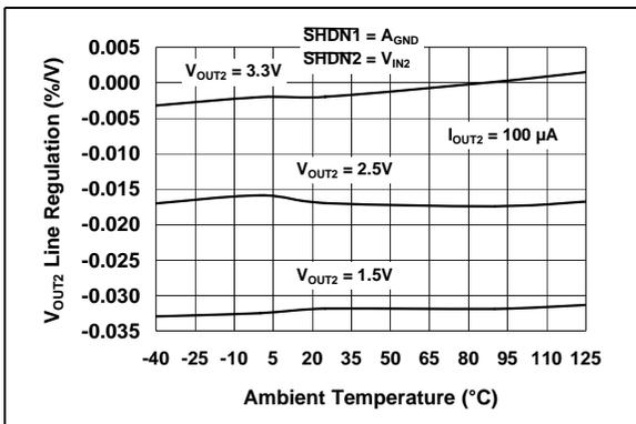
**FIGURE 2-27:**  $V_{OUT2}$  Line Regulation vs. Ambient Temperature.
