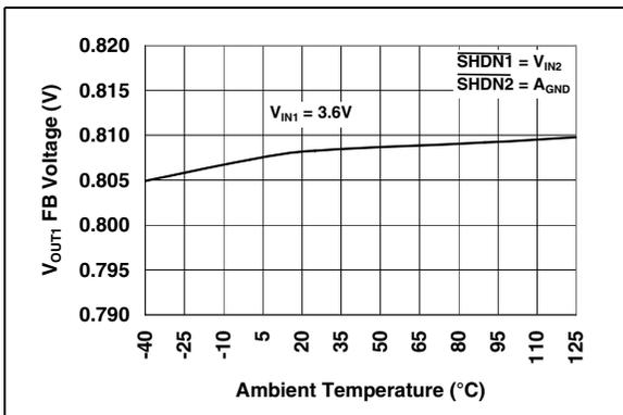
**FIGURE 2-15:**  $V_{OUT1}$  Adjustable Feedback Voltage vs. Ambient Temperature.
