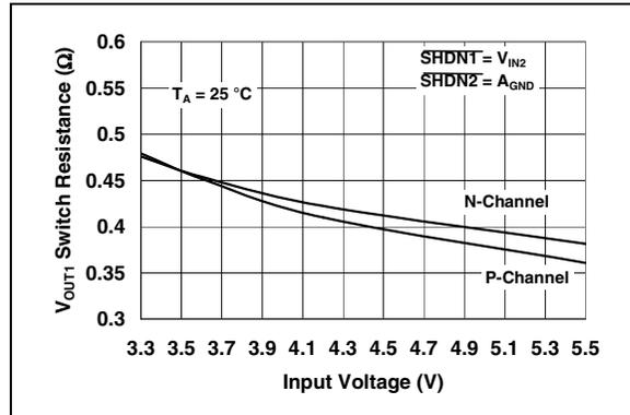
**FIGURE 2-16:**  $V_{OUT1}$  Switch Resistance vs. Input Voltage.
