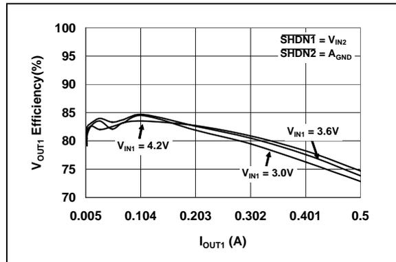
**FIGURE 2-5:**  $V_{OUT1}$  Output Efficiency vs.  $I_{OUT1}$  ( $V_{OUT1} = 1.2\text{V}$ ).
