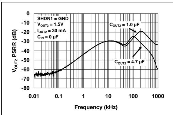
**FIGURE 2-33:**  $V_{OUT2}$  Power Supply Ripple Rejection vs. Frequency.
