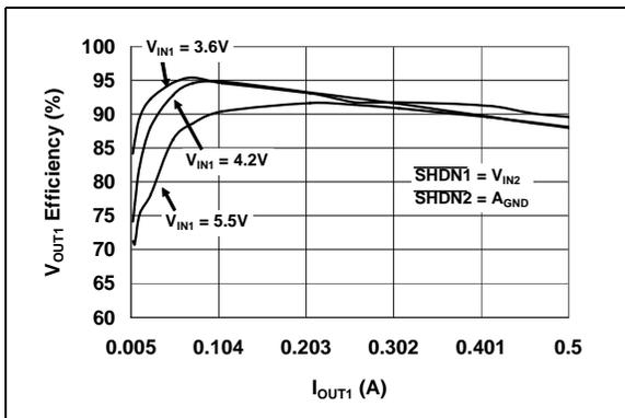
**FIGURE 2-9:**  $V_{OUT1}$  Output Efficiency vs.  $I_{OUT1}$  ( $V_{OUT1} = 3.3V$ ).
