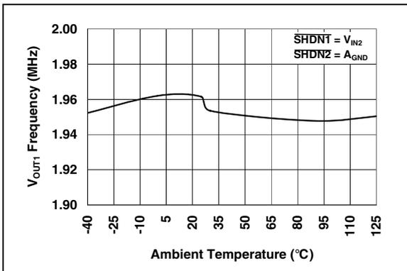
**FIGURE 2-14:**  $V_{OUT1}$  Switching Frequency vs. Ambient Temperature.
