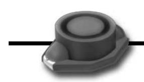
The RL-3316-S Series offers shielded surface mount power inductors in an extremely small flat top package. They have a footprint of .370" x .510" and are low cost with high energy storage. Designed to withstand solder flow, reflow and wave soldering applications. Available in 11 values with inductance ratings from 1.0 $\mu$ H to 47 $\mu$ H and currents up to 5.0 Amps
