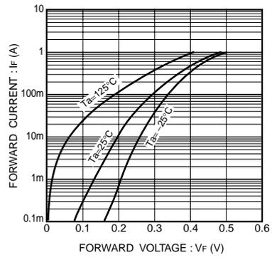
Fig.8 Forward characteristics
