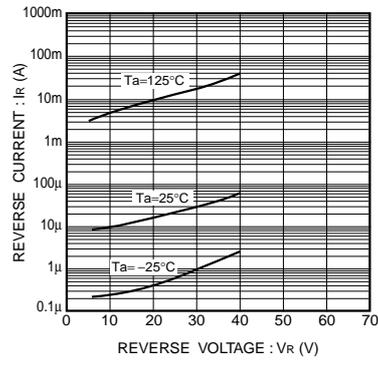
Fig.9 Reverse characteristics
