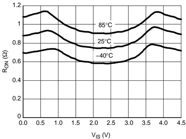
Figure 11. On-Resistance vs. Input Voltage
