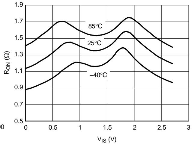
Figure 10. On-Resistance vs. Input Voltage
