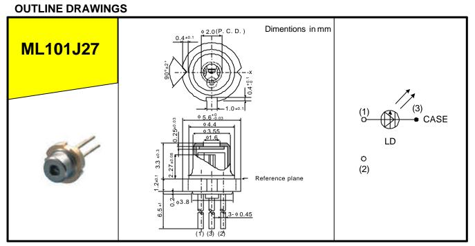
There is no model with a monitor photo diode in ML1XX27 series.
