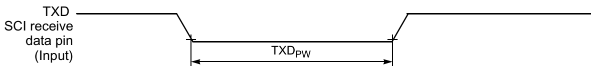
Figure 10-17 TXD Pulse Width
