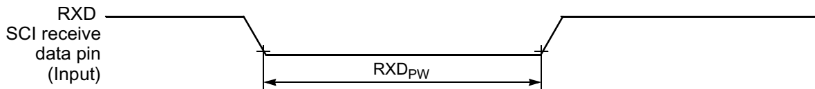
Figure 10-16 RXD Pulse Width
