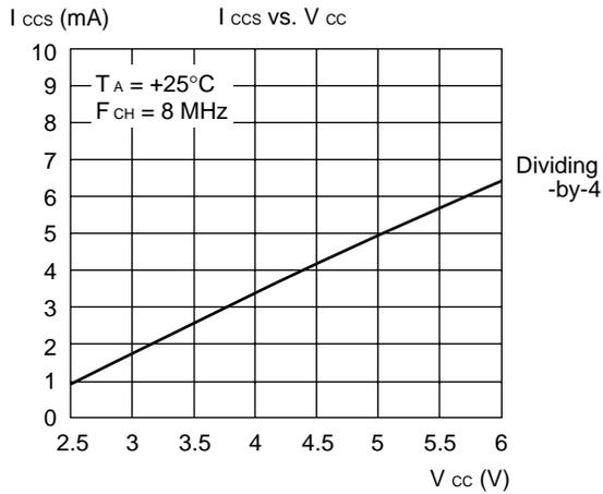
Characteristics of Current Consumption in the Subclock Operation
