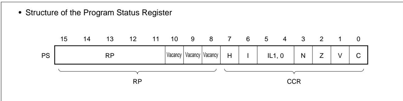
The RP indicates the address of the register bank currently in use. The relationship between the pointer contents and the actual address is based on the conversion rule illustrated below.
