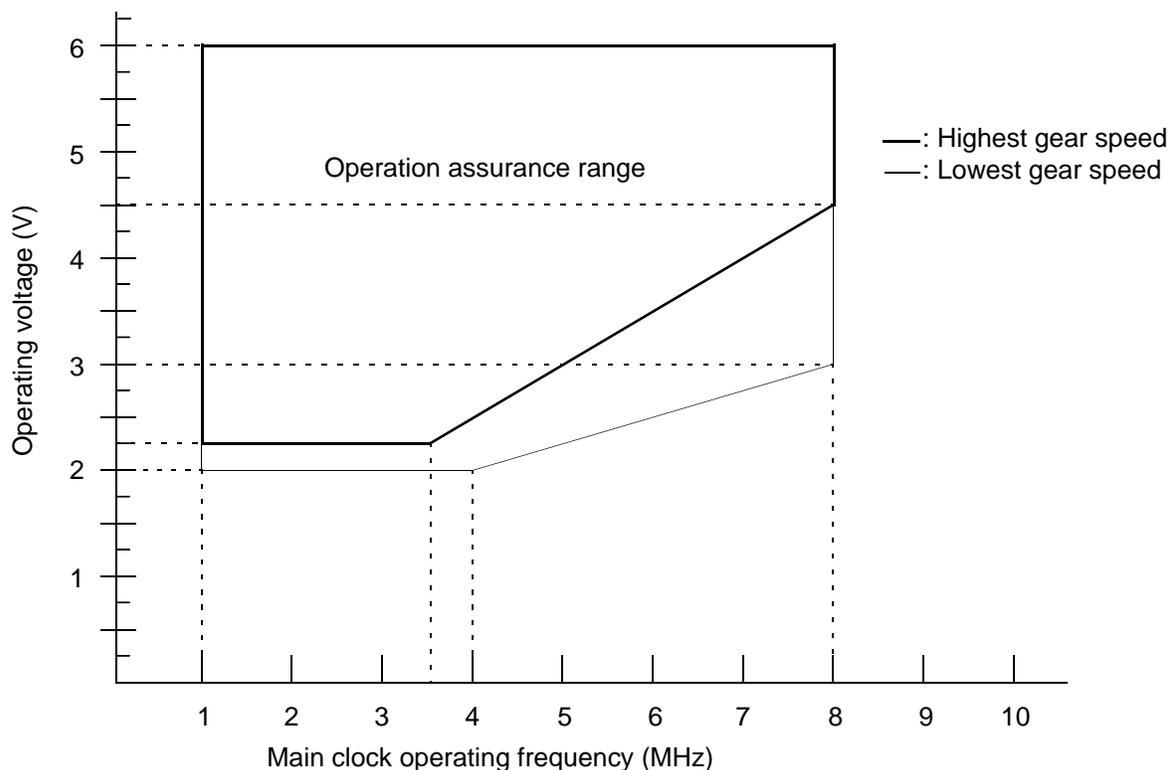
**WARNING:** The recommended operating conditions are required in order to ensure the normal operation of the semiconductor device. All of the device's electrical characteristics are warranted when the device is operated within these ranges.
