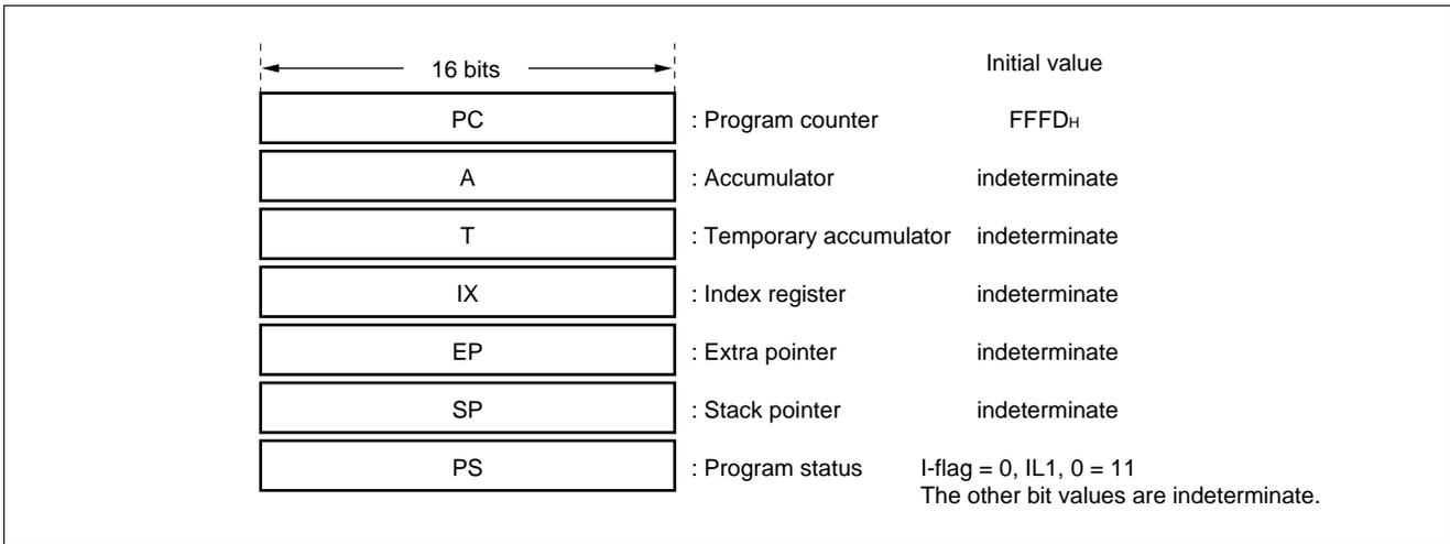
The PS can further be divided into higher 8 bits for use as a register bank pointer (RP) and the lower 8 bits for use as a condition code register (CCR) (see the diagram below).
