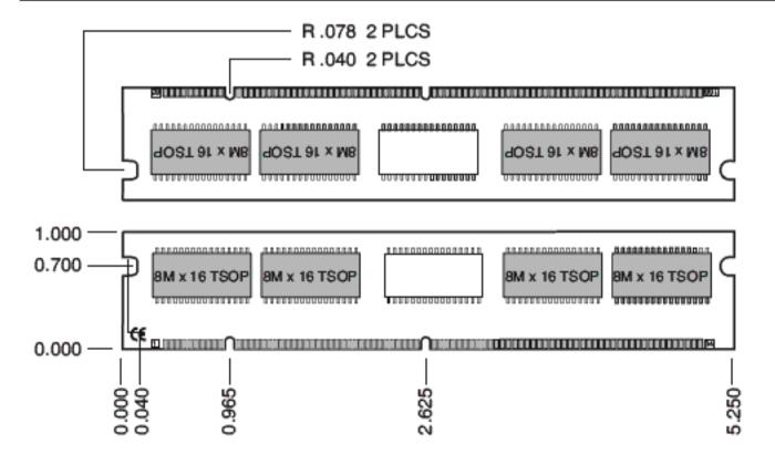
Figure 1: KVR100X64C2L/128 168-Pin SDRAM Module
