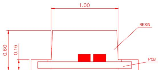
For reflow soldering
