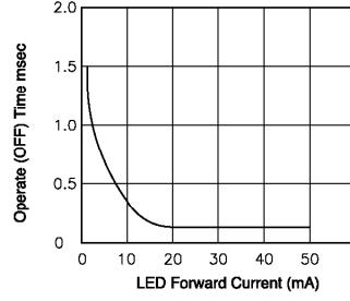
**Fig.11** LED forward current vs. reverse time
