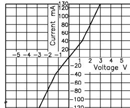
**Fig.9** Off state leakage current
