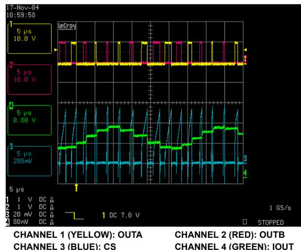
FIGURE 6. DYNAMIC BEHAVIOR OF CS vs IOUT
