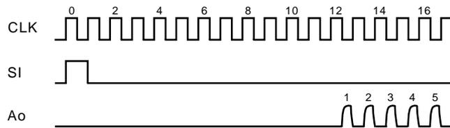
Note) The CLK section area which is over the effective pixel numbers (Output blank part) cannot be used as the analog Output standard level.
