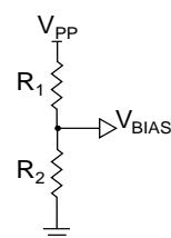
$V_{PP}$  can be used with a voltage divider to get  $V_{BIAS}$  or a separate voltage supply can be used for  $V_{BIAS}$ .
