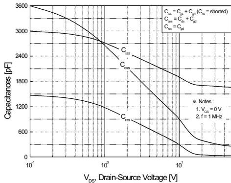
Figure 5. Capacitance Characteristics
