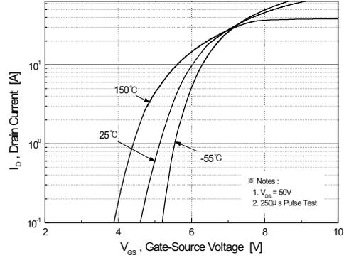
Figure 2. Transfer Characteristics
