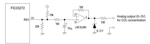
Figure 7 - CO2 concentration signal circuit
