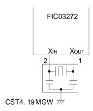
Figure 10 - Clock signal generator circuit
