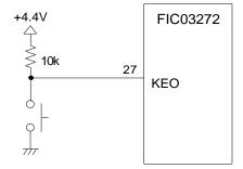
Figure 9 - Manual benchmark reset circuit
