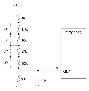
Figure 11 - Damper control signal threshold circuit
