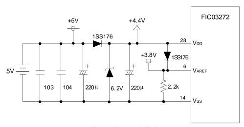
Figure 5 - Power supply circuit
