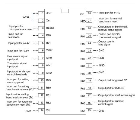
Figure 1 - Pin arrangement for FIC03272
