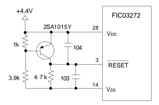
Figure 6 - Reset circuit
