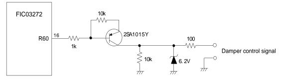
Figure 8 - Damper control circuit
