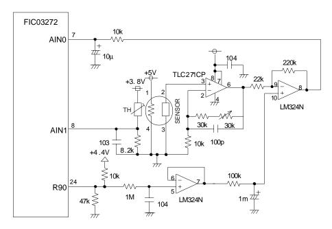
Figure 4 - Circuit for driving sensor and processing sensor signal
