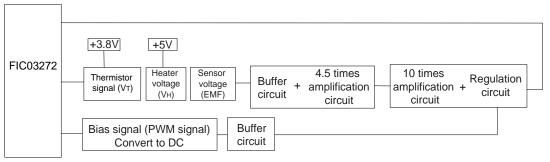
Figure 3 - Block diagram for driving sensor and processing sensor signal
