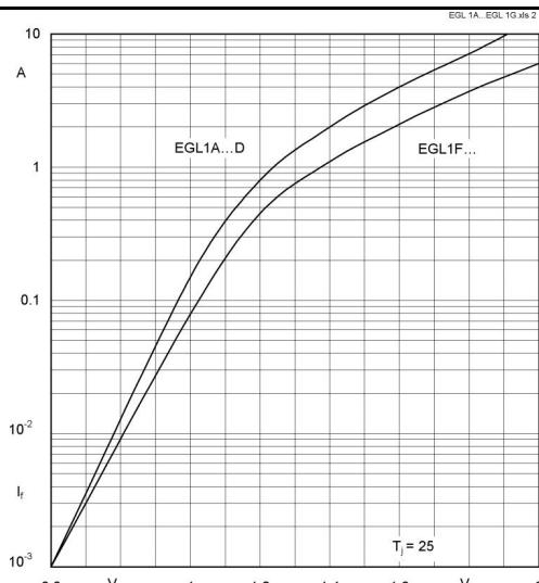
Fig. 1 Forward characteristic ( typical values )
