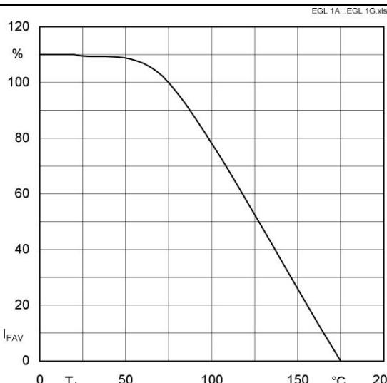
Fig. 2 Rated forward current vs. temp. of the terminals<sup>4)</sup>
