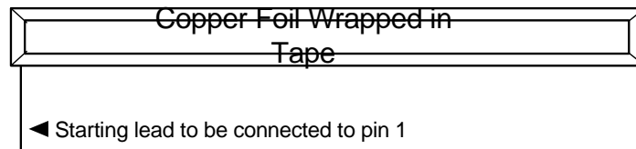
Figure 5 – Copper Foil preparation for winding 3.
