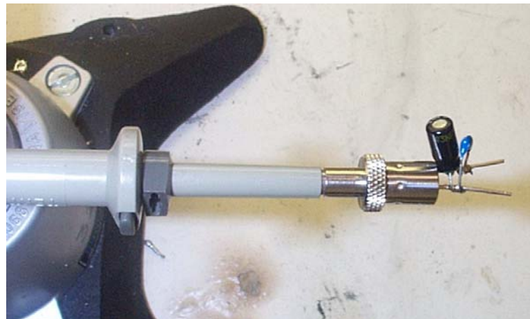
Figure 17 – Oscilloscope Probe with Probe Master 5125BA BNC Adapter. (Modified with wires for probe ground for ripple measurement, and two parallel decoupling capacitors added)
