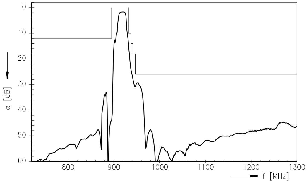
Transfer function (pass band,  $25 \pm 10 \text{ }^\circ\text{C}$ )
