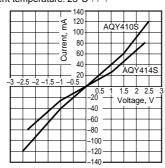
9. Off state leakage current Measured portion: between terminals 3 and 4;
