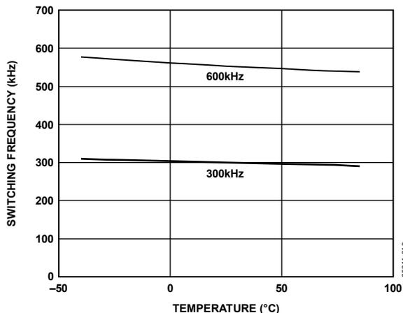
Figure 9. Switching Frequency vs. Temperature
