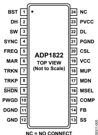
Figure 4. Pin Configuration
