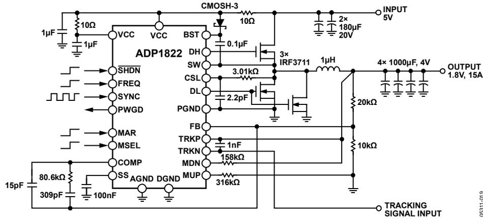
Figure 20. Typical Application Circuit, 5 V Input
