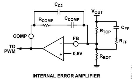
Figure 19. Compensation Using Feed-Forward
