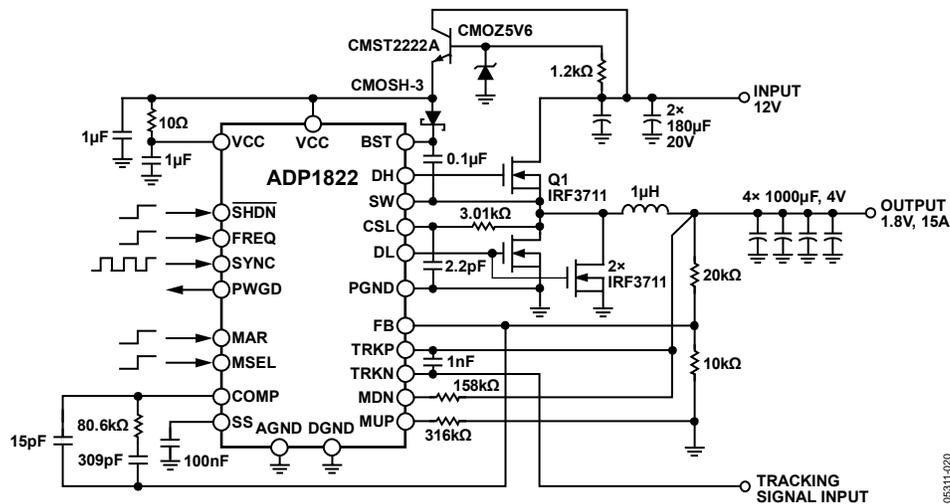
Figure 21. Typical Application Circuit, 12 V Input
