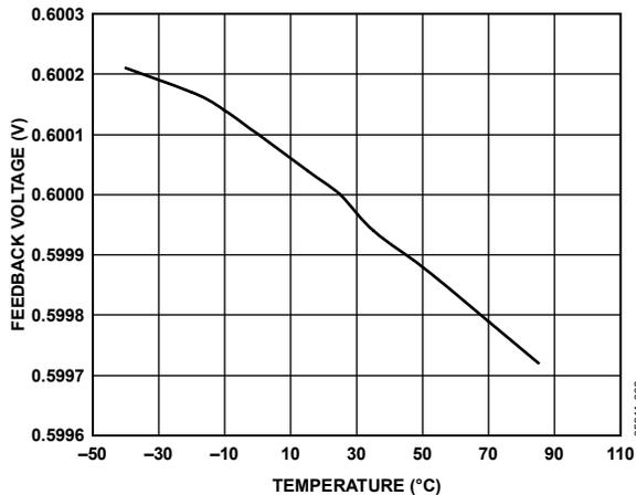
Figure 8. FB Regulation Voltage vs. Temperature
