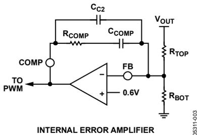
Figure 18. Compensation Using the ESR Zero
