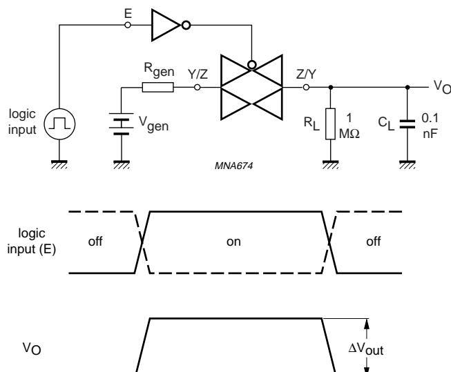
Fig.21 Charge injection test.
