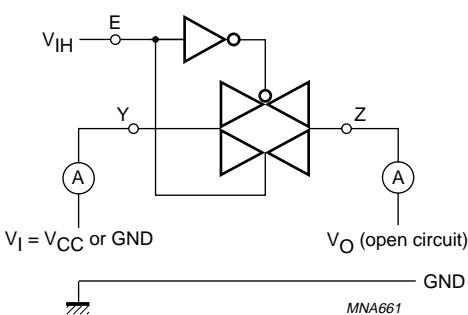
Fig.6 Test circuit for measuring ON-state current.
