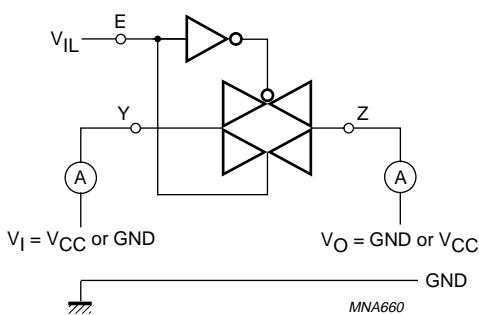
Fig.5 Test circuit for measuring OFF-state current.
