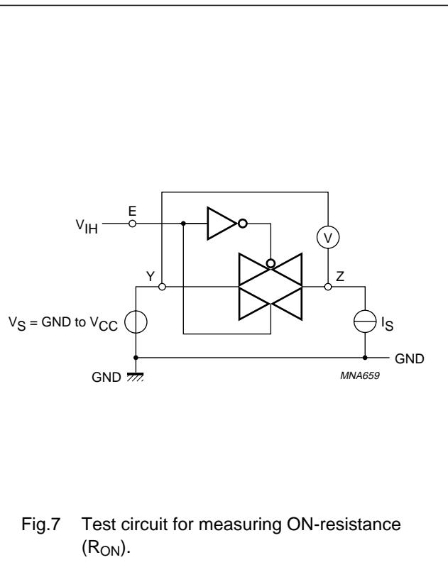
Fig.7 Test circuit for measuring ON-resistance ( $R_{ON}$ ).
