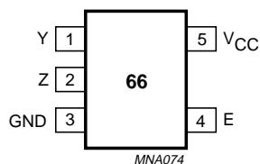
Fig.1 Pin configuration.
