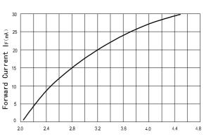
Forward Current VS Forward Voltage
