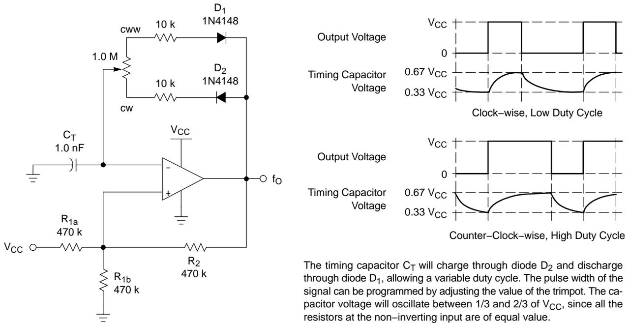
Figure 35. Variable Duty Cycle Pulse Generator
