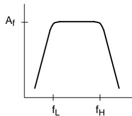
$$f_L = \frac{1}{2\pi R_1 C_1} \approx 200 \text{ Hz}$$
