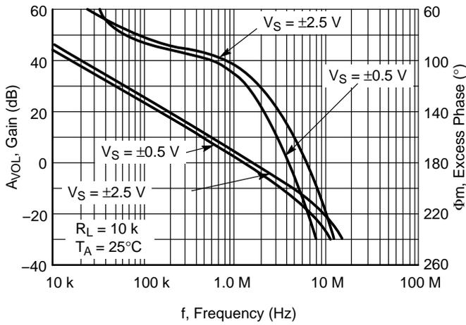
Figure 20. Voltage Gain and Phase vs. Frequency
