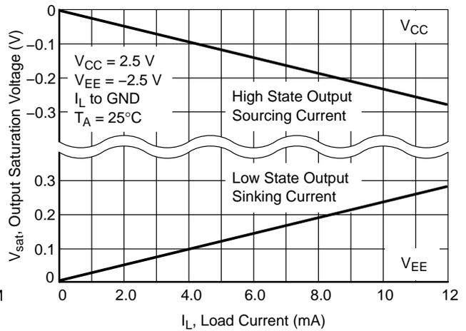
Figure 3. Split Supply Output Saturation vs. Load Current
