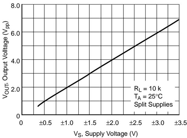
Figure 24. Output Voltage Swing vs. Supply Voltage
