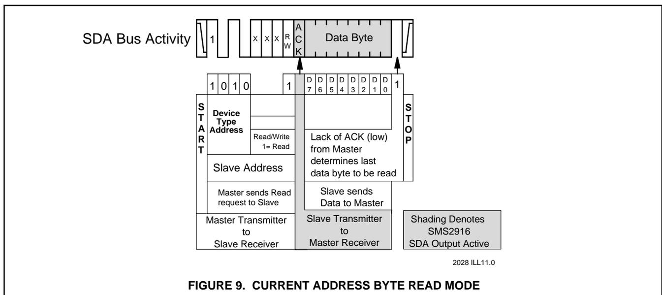
**FIGURE 9. CURRENT ADDRESS BYTE READ MODE**
