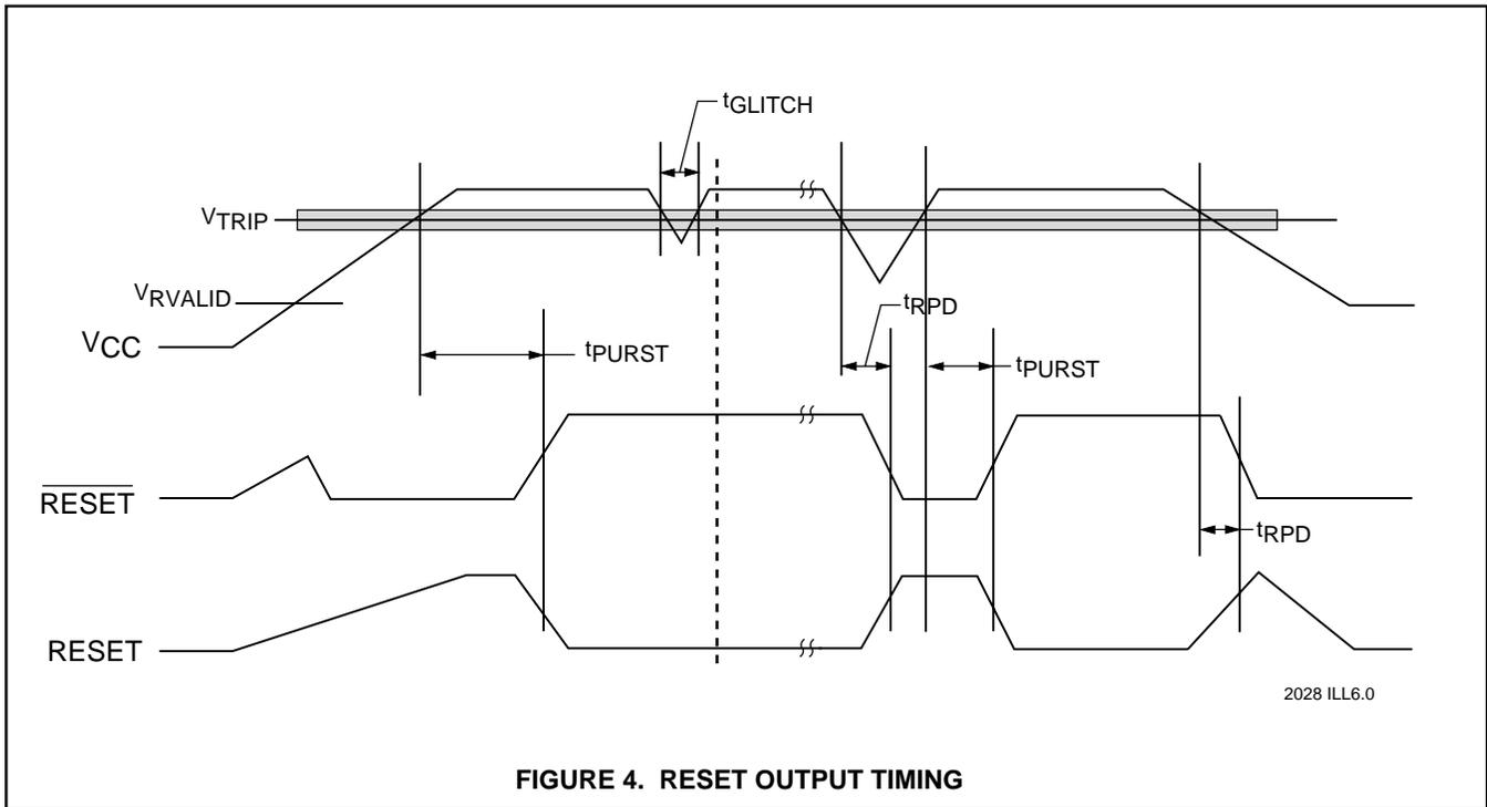
**FIGURE 4. RESET OUTPUT TIMING**
