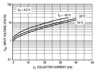
Figure 5. Input Voltage versus Output Current
