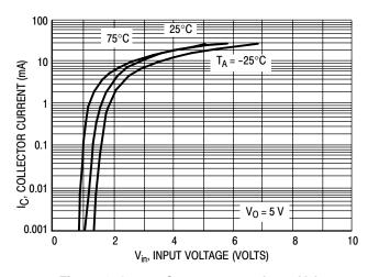
Figure 4. Output Current versus Input Voltage
