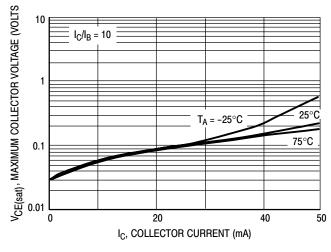
Figure 1. V<sub>CE(sat)</sub> versus I<sub>C</sub>
