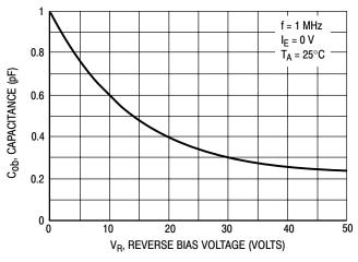
Figure 3. Output Capacitance
