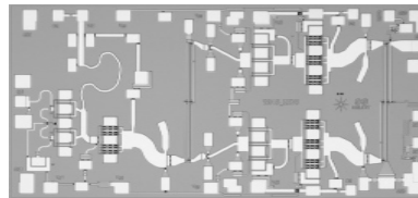
Chip Size: 2730 x 1300 \mu\text{m} (108 x 51.6 mils) Chip Size Tolerance: \pm 10 \mu\text{m} ( \pm 0.4 mils) Chip Thickness: 100 \pm 10 \mu\text{m} (4 \pm 0.4 mils) Pad Dimensions: 80 x 80 \mu\text{m} (2.95 \pm 0.4 mils)
