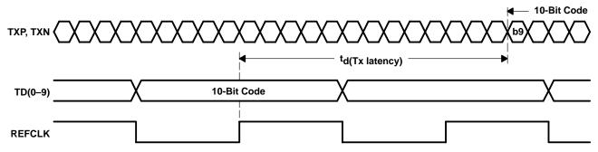
Figure 1. Transmitter Latency Full Rate Mode
