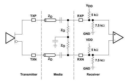
Figure 11. High-Speed I/O AC-Coupled Mode
