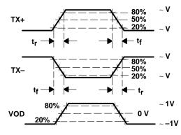
Figure 7. Differential and Common-Mode Output Voltage Definitions
