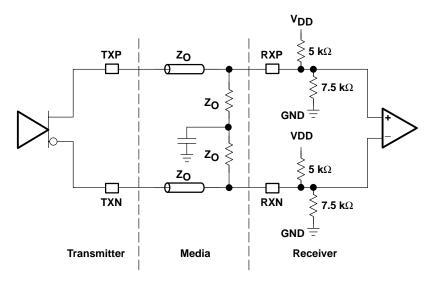
Figure 10. High-Speed I/O Directly-Coupled Mode
