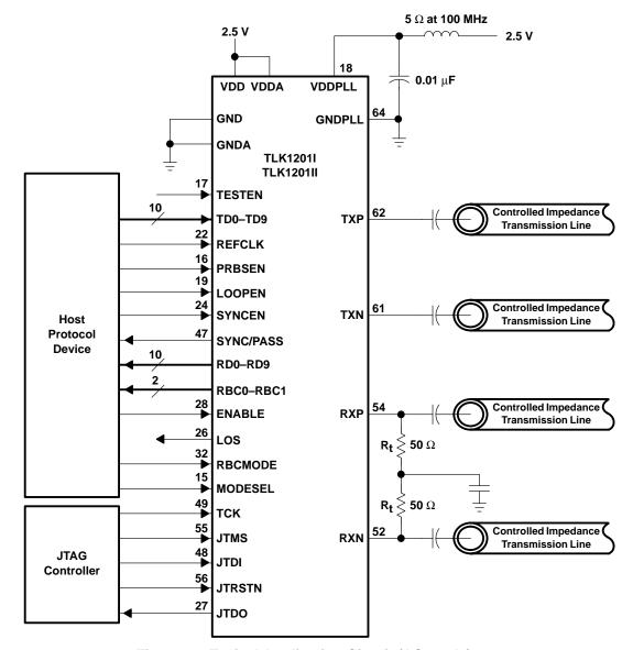
Figure 12. Typical Application Circuit (AC mode)
