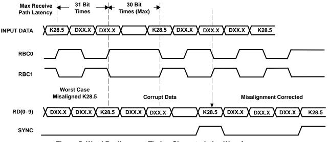
Figure 5. Word Realignment Timing Characteristics Waveforms
