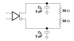
Figure 8. Transmitter Test Setup
