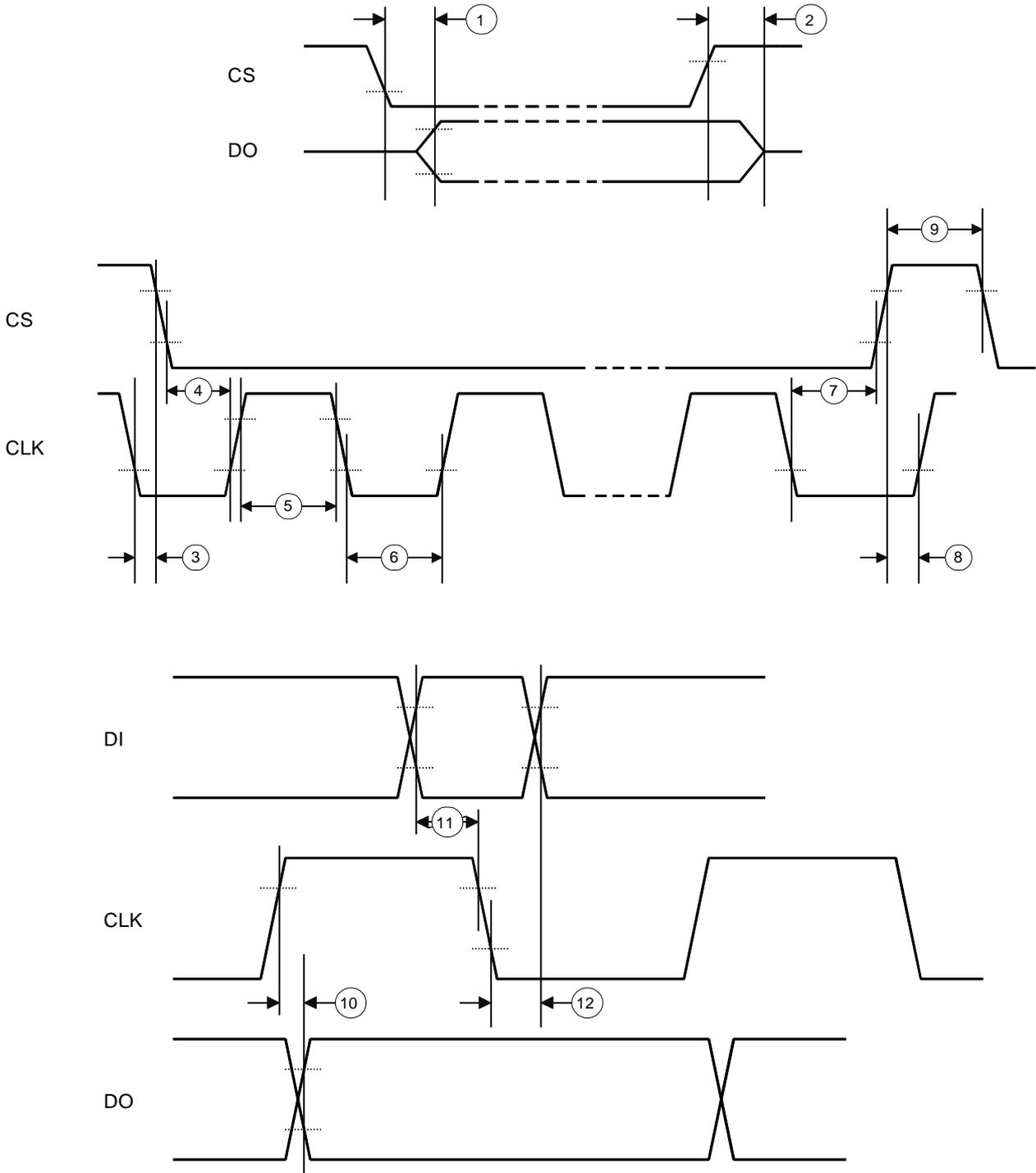
Inputs DI, CLK, CS: High level =  $0.7 \times V_{CC}$ , low level =  $0.3 \times V_{CC}$
