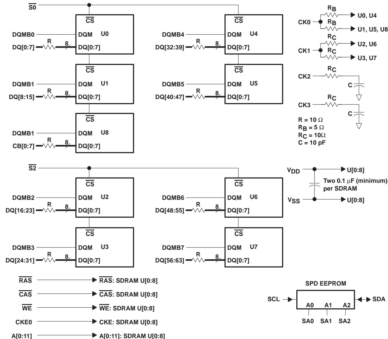
functional block diagram for the TM4SR72EPU
