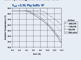
Note: A All data listed in the above graphs has been developed from actual products tested at 25°C. This data is considered typical data for the ISR.
