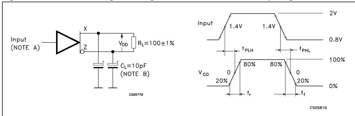
Note A: All input pulse are supplied by a generator having the following characteristics:  $t_r$  or  $t_f \leq 1\text{ns}$ , pulse repetition rate (PRR) = 50Mpps, pulse width =  $10 \pm 0.2\text{ns}$ .
