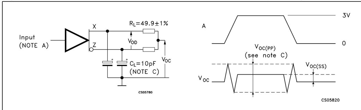
Note A: All input pulse are supplied by a generator having the following characteristics:  $t_r$  or  $t_f \leq 1$  ns, pulse repetition rate (PRR) = 50Mpps, pulse width =  $10 \pm 0.2$  ns.
