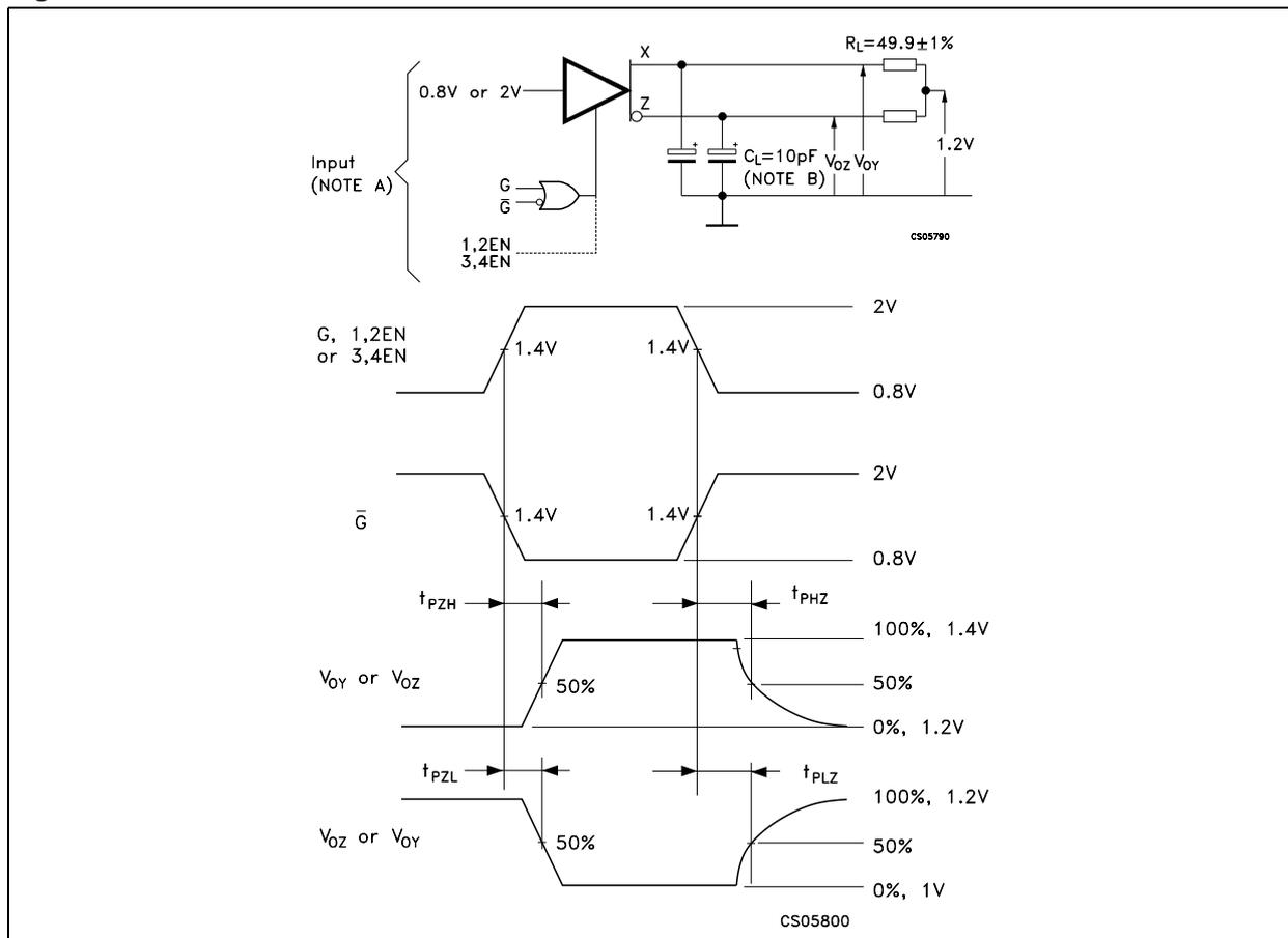
Note A: All input pulse are supplied by a generator having the following characteristics:  $t_r$  or  $t_f \leq 1$  ns, pulse repetition rate (PRR) = 0.5Mpps, pulse width =  $500 \pm 10$  ns.
