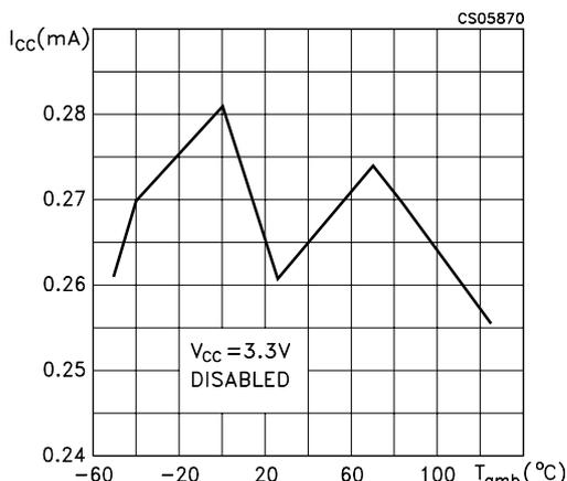
**Figure 8. Supply Current vs Temperature**
