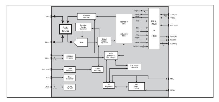
The Broadcom BCM5228 is a single-chip device containing eight independent Fast Ethernet transceivers. Each performs all the physical layer functions for 100BASE-TX full-duplex or half-duplex Ethernet on Category 5 UTP cable and 10BASE-T full-duplex or half-duplex Ethernet on Category 3, 4, or 5 UTP cable.
