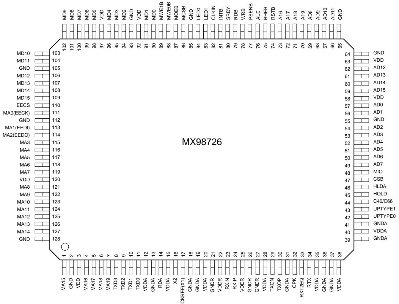
**2.1 Pin Description : ( all internal pull-up resistor is 168K ohm, pull-down is 70k ohm )**
