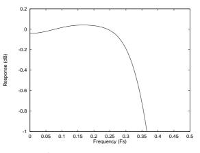
Figure 10 DAC Digital Filter Ripple -192kHz
