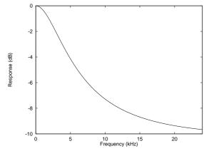
Figure 15 De-Emphasis Frequency Response (48kHz)
