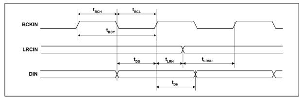
Figure 2 Digital Audio Data Timing
