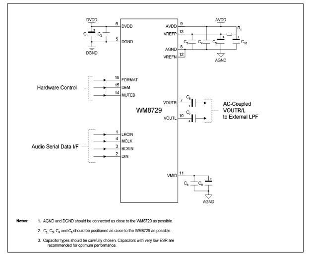
Figure 17 External Component Diagram
