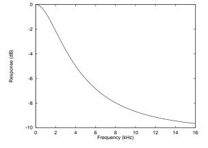
Figure 11 De-Emphasis Frequency Response (32kHz)
