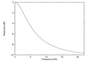
Figure 13 De-Emphasis Frequency Response (44.1kHz)
