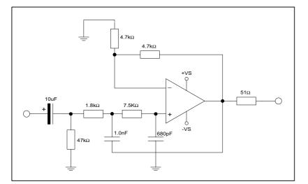
Figure 18 Recommended Low Pass Filter (Optional)
