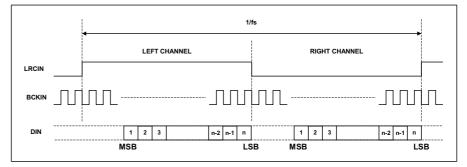
Figure 3 Right Justified Mode Timing Diagram
