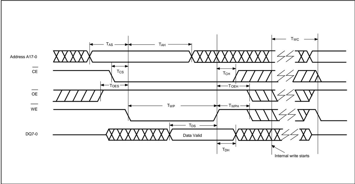
**CE Controlled Write Cycle Timing Diagram**
