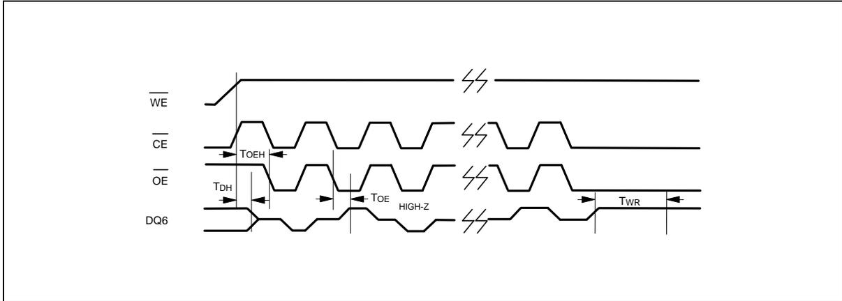
**Page Write Timing Diagram Software Data Protection Mode**
