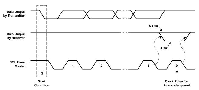
Figure 3. Acknowledgment on I<sup>2</sup>C Bus
