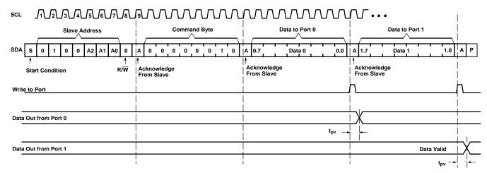
Figure 6. Write to Output Port Registers
