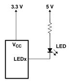
Figure 17. Device Supplied by Lower Voltage
