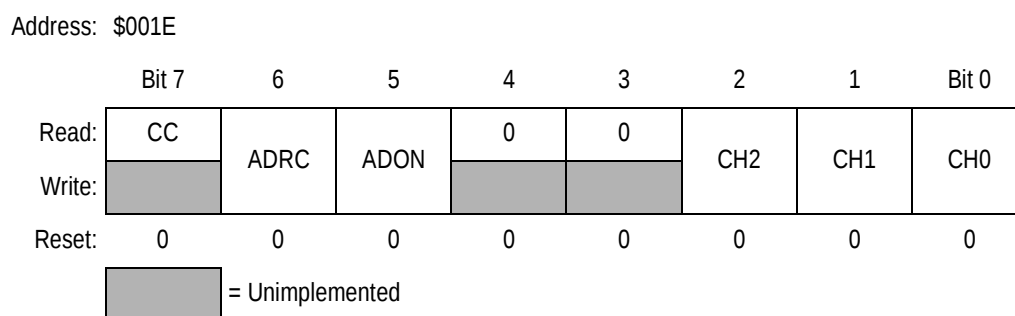
Figure 9-1. A/D Status and Control Register (ADSC)
