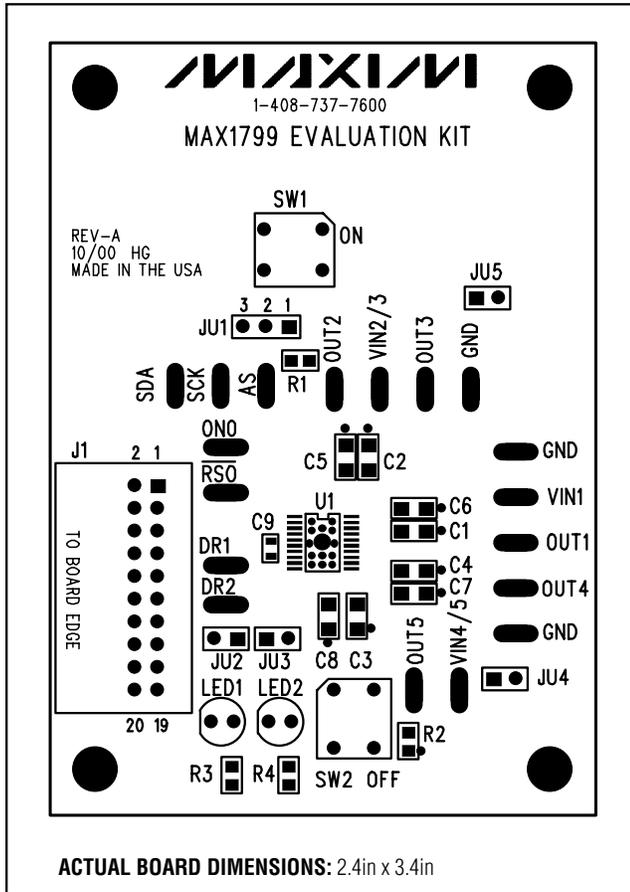
Figure 3. MAX1799 EV Kit Component Placement Guide—Component Side
