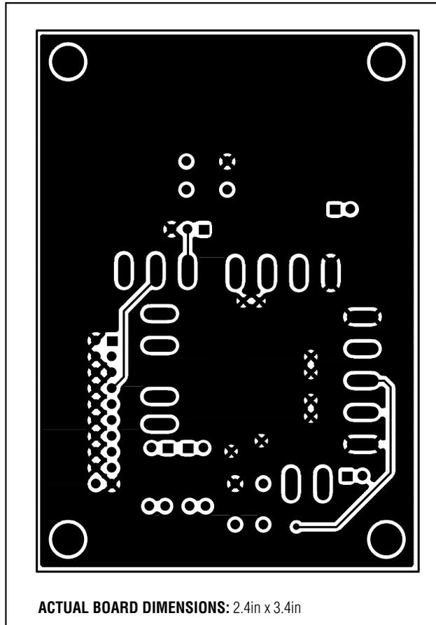
Figure 5. MAX1799 EV Kit PC Board Layout—Solder Side
