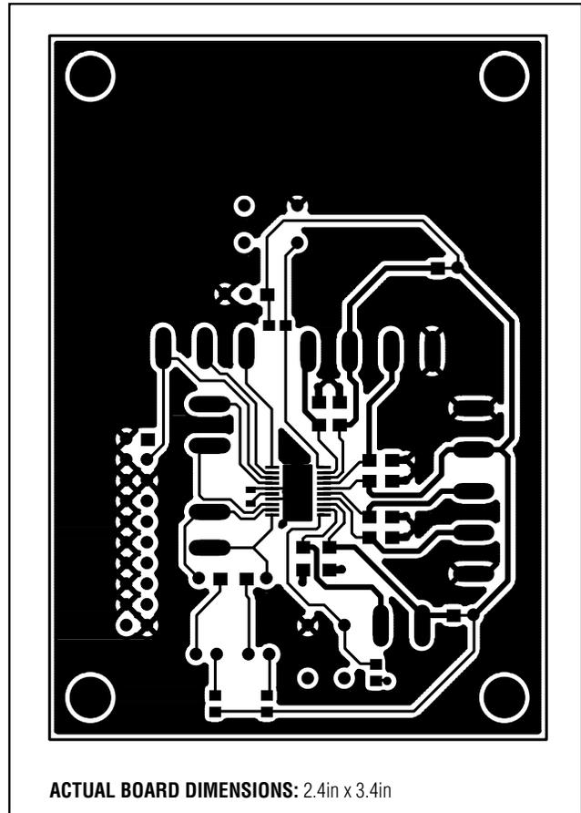
Figure 4. MAX1799 EV Kit PC Board Layout—Component Side
