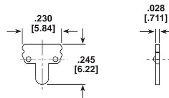
When ordering polarizing keys individually, specify Model Number: PK-7 between contacts. Hand insertion tool, TPK-7, provided on request.
