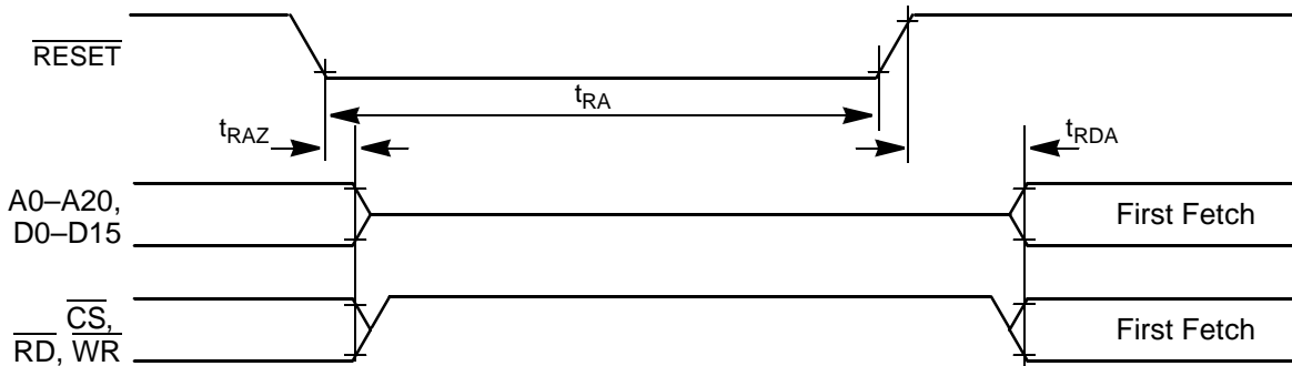
Figure 12. Asynchronous Reset Timing
