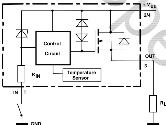
1) For 12 V applications only. Reverse load current only limited by connected load.
