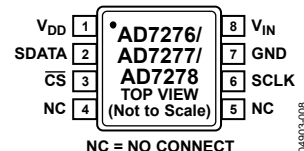
Figure 9. 8-Lead MSOP Pin Configuration
