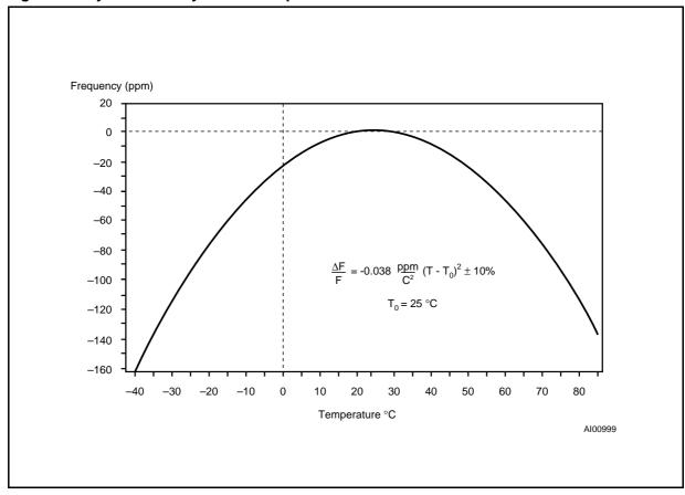
Figure 14. Crystal Accuracy Across Temperature
