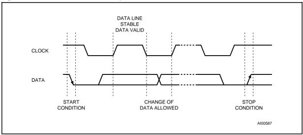
Figure 6. Serial Bus Data Transfer Sequence
