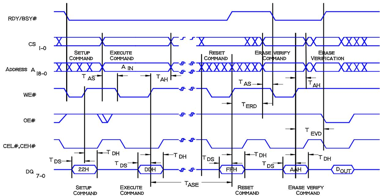
**Figure 9: Sector Erase Timing Diagram**
