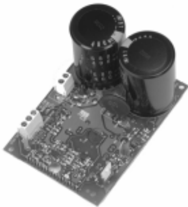
Figure 3. IRPT1058D Driver-Plus Board
